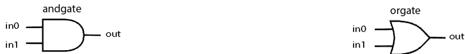
Figure 2: an AND gate and an OR gate. The Verilog code is included above the gate diagrams, and the representative diagram is included below. The inputs, output, and gate names are labeled.
