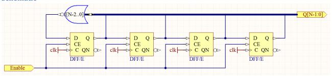
Note: The NOR gate restarts the cycle when the hot bit is at the end of the ring. This structure obviates the need for a reset signal and is self-cleaning.
