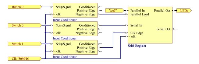
The Parallel Load feature is tied to the constant value of 0xA5, and is activated when Button 0 is pressed.
