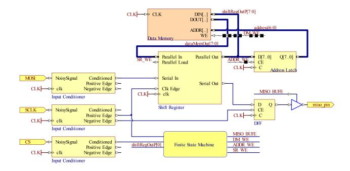
This is a \_recommended\_ schematic for the SPI Memory. The next few pages provide additional scaffolding for this design route, but you may choose to implement your SPI Memory by any means you find appropriate. Stubbed signals are controlled by the Finite State Machine. You may require additional signals as inputs to the FSM. System Clock routed as a net label for clarity.
