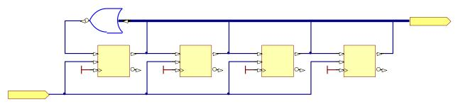
Note: The NOR gate restarts the cycle when the hot bit is at the end of the ring. This structure obviates the need for a reset signal and is self-cleaning.
